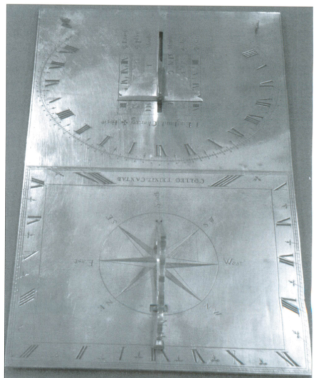
Fig.5. John England's 1703 analematic dial with the elliptical dial furthest from the observer and (inset), the scales along the base of its sliding vertical gnomon.
